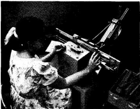
The Kingman Machine, above, is another device born and built at -hp- to make possible faster manufacturing at lower cost. Named for the -hp- engineer who "imageered" it, it mass-produces terminal boards.
