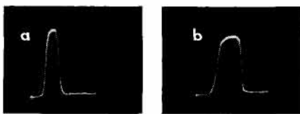
Figure 1. (a) 0.01 \mu sec pulse through -hp- 460B Amplifier. (b) 0.02 \mu sec pulse through 3 amplifiers in cascade.
